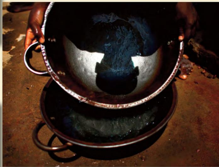
To extract gold from the raw ore, workers must first crush the ore, then wash and strain it through car floor mats. Finally the slurry is ground together by hand with a silvery glob of mercury in large metal wash basins, like the one used here at a gold processing site in Dareta, Nigeria.
