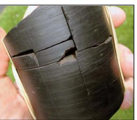
A section of Marcellus shale that's been fracked. Deep under the earth, fracking opens fissures in the shale that allow oil and gas to seep into the hole left behind from drilling. The gas is then pumped up and out of the well.
